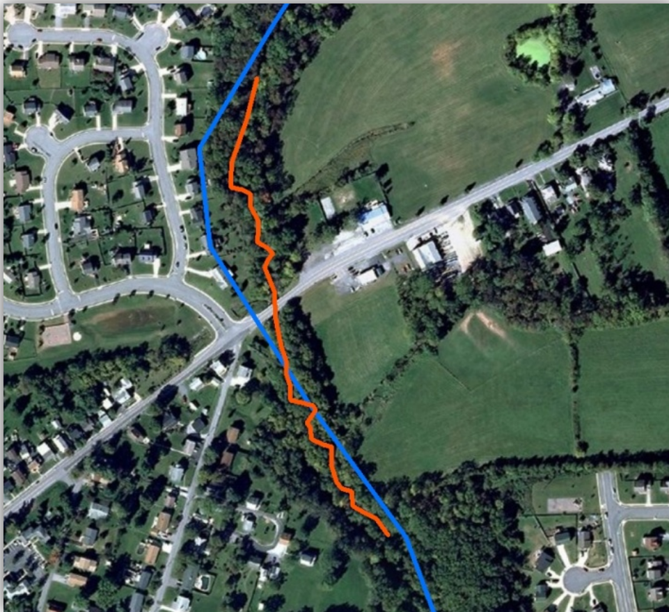
Figure A5-11: Comparison of computed reach length (blue) to the stream thalweg (red)
